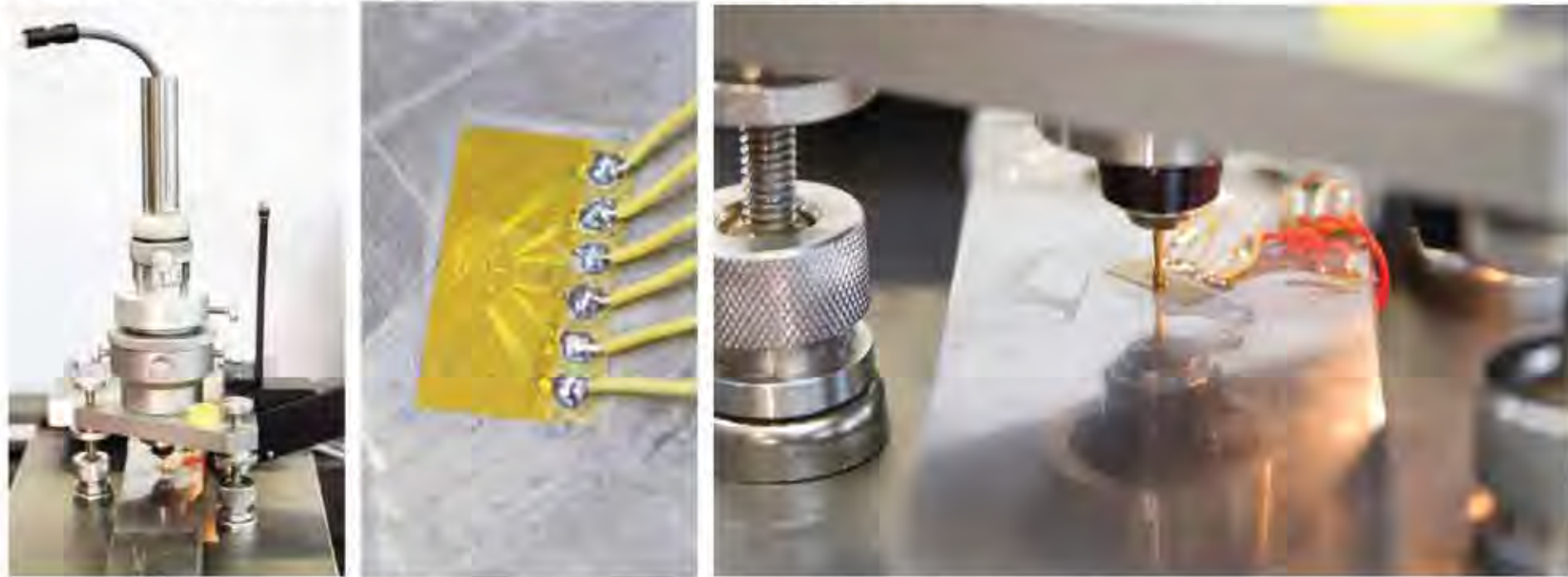
Fig. 1 - From the left: drilling equipment, strain-gage rosette, setup configuration.
